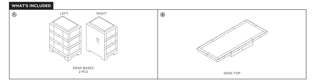
Carefully remove both bases (A) from their boxes and arrange them side by side, about 2 feet apart. The single mirror sides of the bases should be facing each other.
